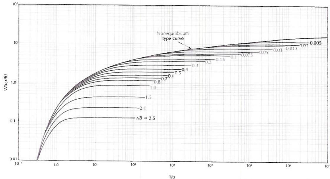
Figure 6. Type curves for aquifers with leaky confining zones.
