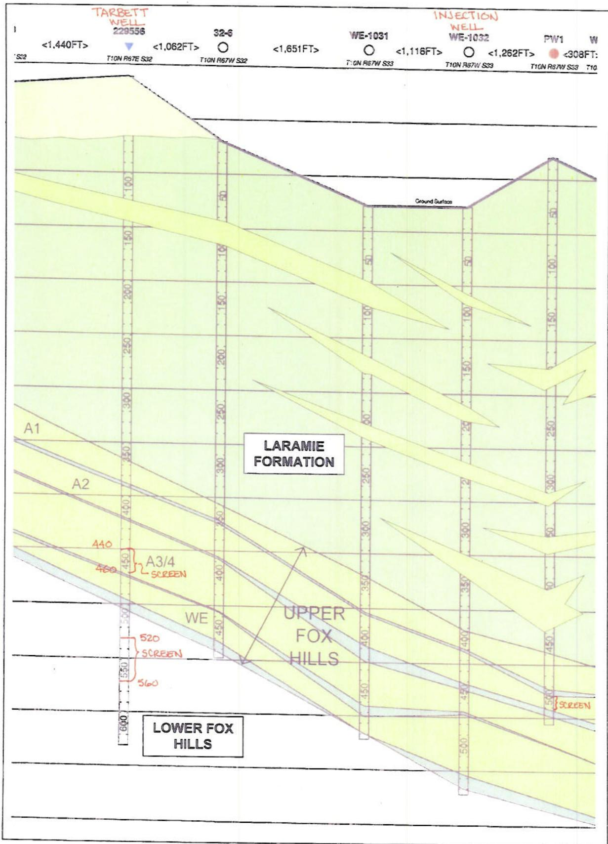
Figure 7b. Cross section showing Tarbett well, the nearest domestic well to the proposed injection well.
