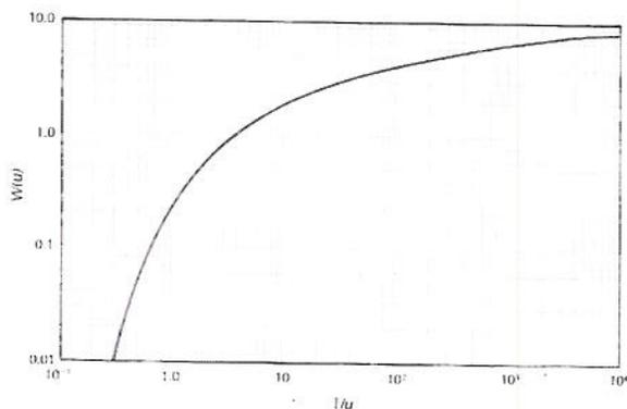
Figure 5a. Theis curve for fully confined aquifers.
